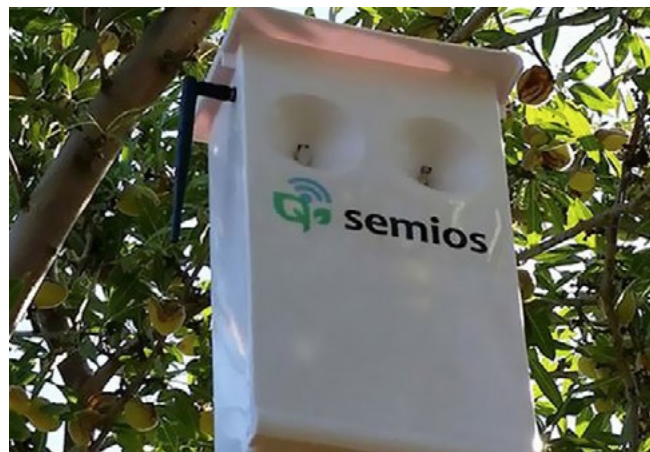
Figure 2: Semios orchard monitoring system has sensors which measure frost, leaf-wetness, soil moisture, and pest pressure and uploads that data to the cloud.
