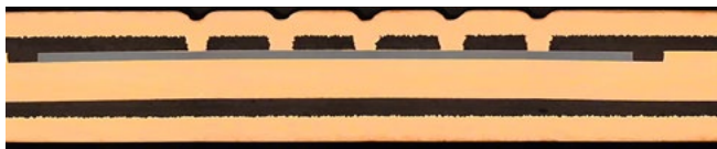
Figure 11: Cross-section of a p 2 Pack with Cu-filled microvias.
